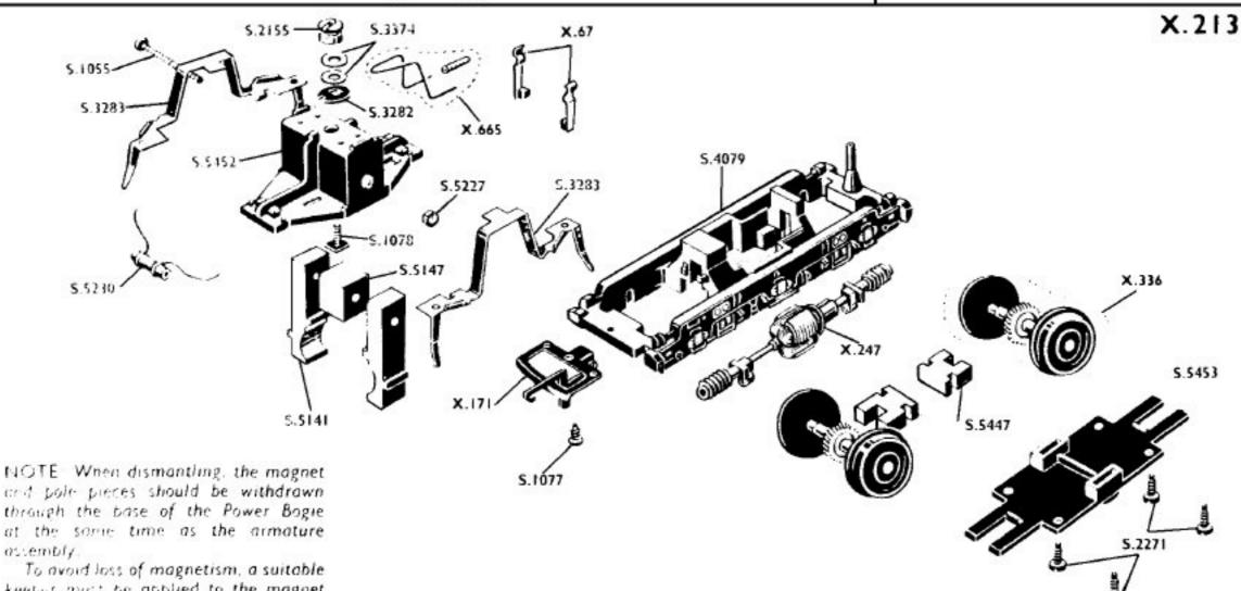
assembly. To avoid loss of magnetism, a suitable keeper must be applied to the magnet before it is separated from the pole Merchi
